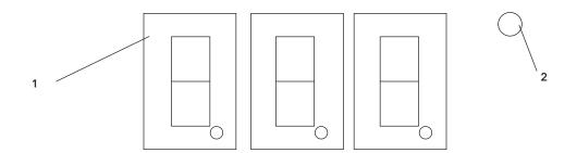
1. When the SET key is pressed, the three nixie tubes show set temperature. This temperature can be adjusted by pressing -or+ key to reach the required value. When the heating control deactivates, the display shows the present temperature.
